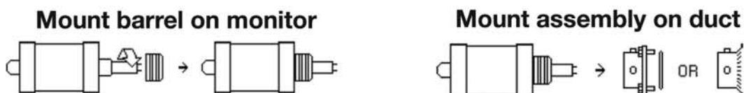
Figure 5: Mount Kit Installation Examples
