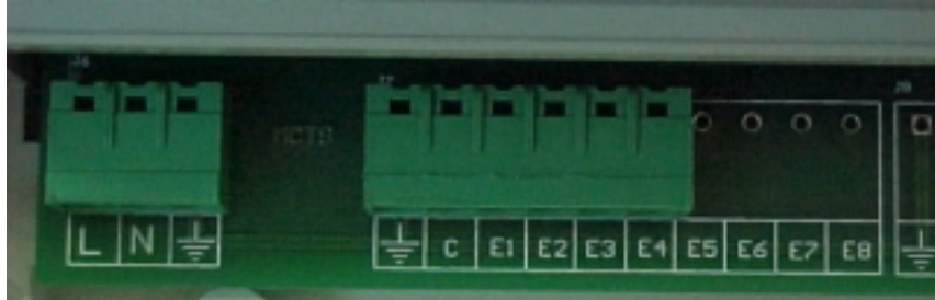
Figure 6 - Output terminals for solenoids
